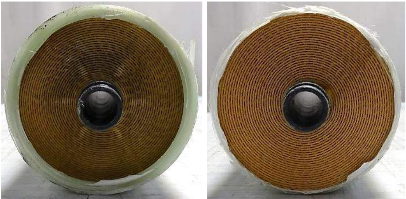
Image of feed scroll end (left) and concentrate scroll end (right) of SN 2190321127
