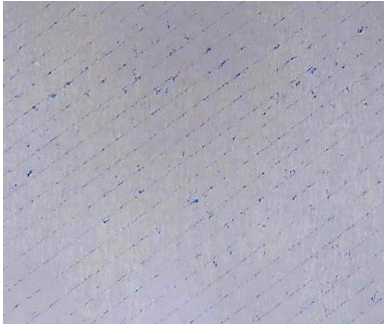
Image of dye uptake on the membrane surface
