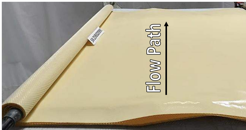
Exposed membrane surface from feed end of SN 2190320991
