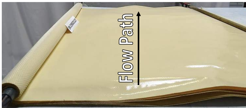
Exposed membrane surface from feed end of SN 2190321127
