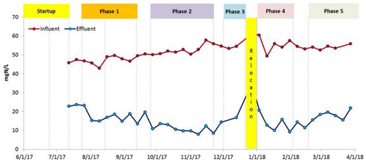
Figure 3. JWPCP Mainstream ANITA Mox Pilot Testing – Influent and Effluent TN during Ambient Temperature Testing
