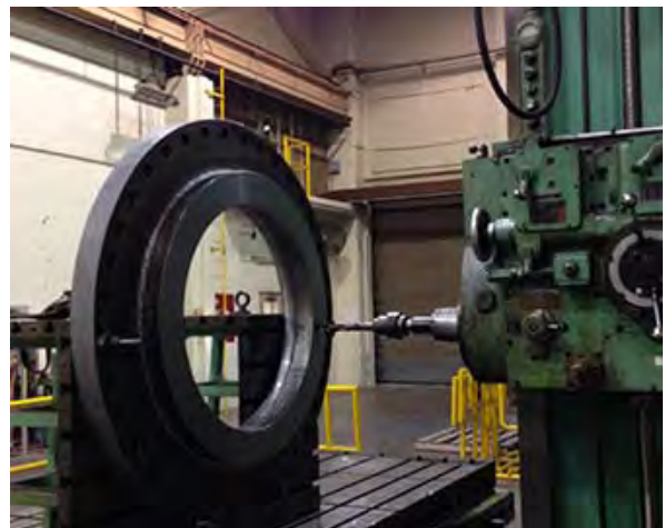
Photo of the 120-inch Froriep Vertical Turning Lathe (above) and the 5-inch G&L Horizontal Boring Mill (below) in the La Verne Machine shop.
