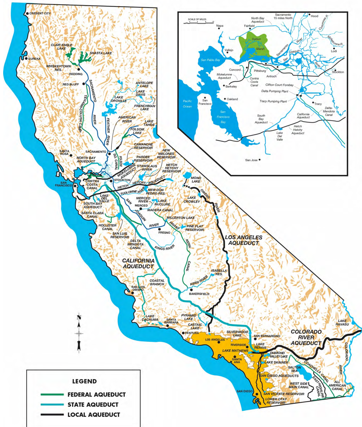
Figure A.2-5 MAJOR WATER CONVEYANCE FACILITIES IN CALIFORNIA
